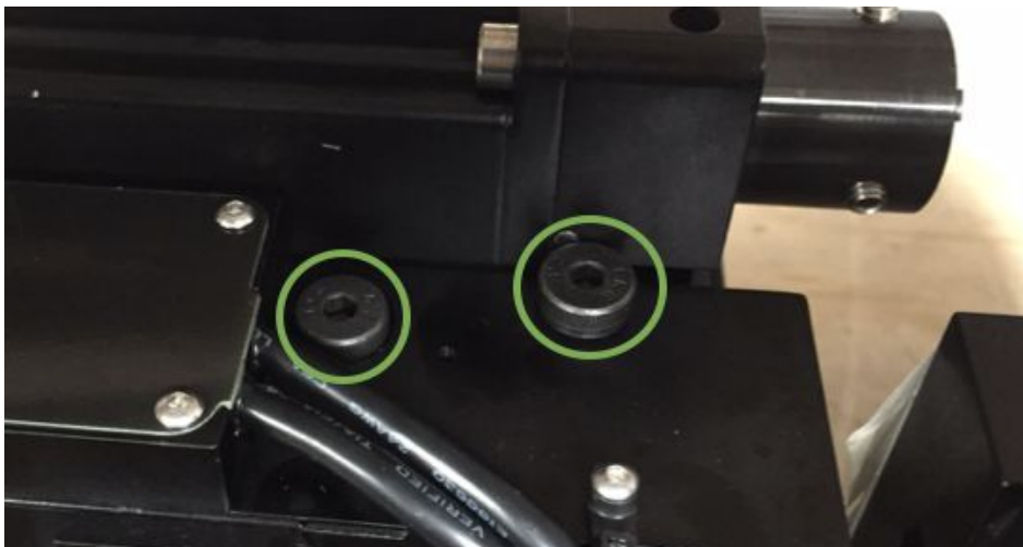
Figure 3: Close up of shipping bolts in green on X-carriage
