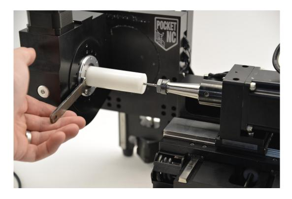
With the material tight and a finger over the E-stop button, press the blinking Start button to let the machine begin cutting the face of the part. From there the program should run smoothly, following the tool paths shown in the simulator. The operator just needs to be ready to stop the machine (finger over E-stop) in case of any of the following:
