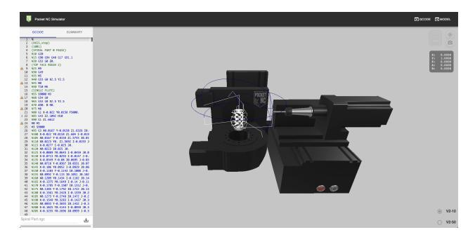
Because this part's G-code has been proven many times, the use of the simulator here is mainly to show the part that will be made and demonstrate how the machine will move. Take note of
