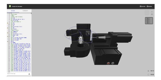
Because this part's G-code has been proven many times, the use of the simulator here is mainly to show the part that will be made and demonstrate how the machine will move. Take note of the first few moves of the machine. If errors do pop up when this G-code is simulated, they will likely be a tool or tool holder issue, so make sure those values and settings are correct.
