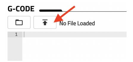
From there, the "Spiral Part" G-code may be selected from its saved location on the computer. The UI will show the progress of the upload as well as produce a notification when the upload is finished.
