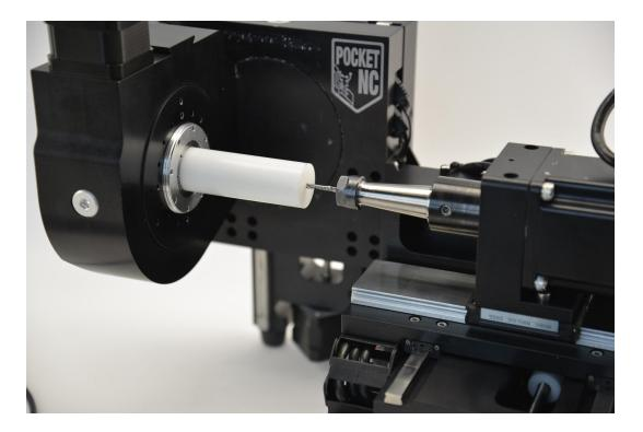
While keeping the material in contact with the tip of the tool, use the ER40 fixture wrench to tighten the top collet ring and secure the material. Shown in the picture below.
