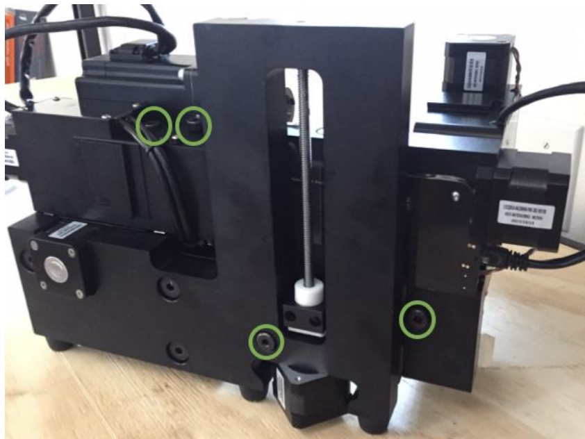
Figure 1: Pocket NC V2 Series all shipping bolt locations shown in green circles.
