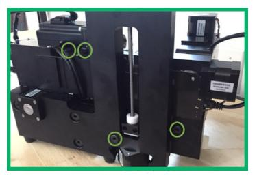
Figure 1: Pocket NC V2 Series all shipping bolt locations shown in green circles.
