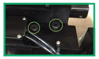
Figure 3: Close up of shipping bolts in green on X-carriage
