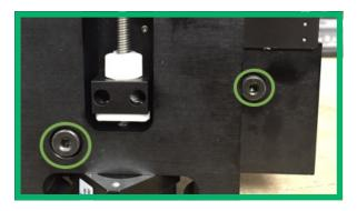
Two of the shipping bolts are located behind the Y-axis, they are shown in green circles in Figure 2. When the user is looking at the back of the machine they are located in the lower-right quadrant of the machine. One of them locks the trunnion housing to the L-bracket and the other locks the A-table to the A-housing.
